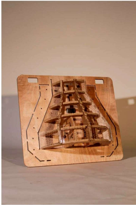
Figure 3. Network-based prototyping design one is a concrete footing formwork designed to improve footing surface finish and column load distribution. Researchers built the mould shown to transfer to a fiberglass boat repair contractor in Tai O Village. The fiberglass contractor will cast a two-part fiberglass mould from this master. Contractors in Tai O can then use the fiberglass mould to cast higher-quality footings. Design, fabrication, and photograph by Daniel Keith Elkin.
